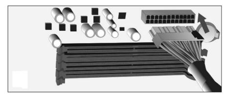
3. Connect the 8-pin or 4+4-pin connector for the CPU. If your motherboard has an 8-pin socket with a cover on some of the openings, we recommend that you remove the cover and use the 8-pin connector.
